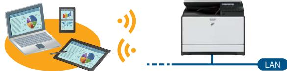
**Access point mode** wirelessly connects a LAN-wired MFD to notebook PCs and other mobile devices without going through a wireless LAN router. The MFD can be accessed via both a wired connection and a wireless connection. Note: External networks cannot be accessed via the MFD. Up to five mobile devices can be wirelessly connected to the MFD at the same time.
