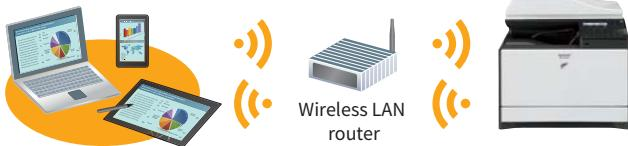
**Infrastructure mode** wirelessly connects the MFD to notebook PCs and other mobile devices via a commercially available wireless LAN router. This ensures convenient access to the MFD even from places where wired LAN is not available.
